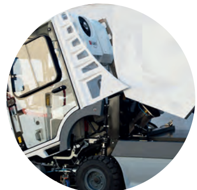
Kippbare Kabine aus Aluminium Aluminum tilting cab
